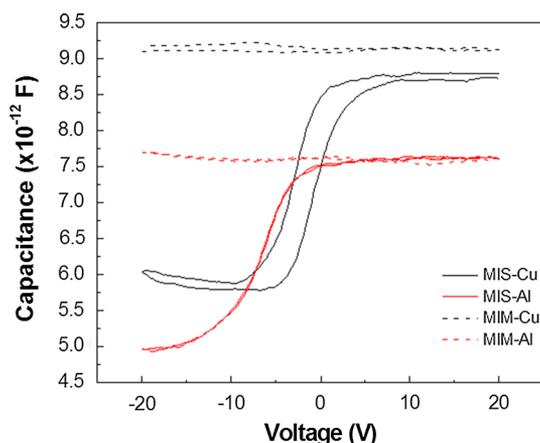
Fig. 2.  $C$ - $V$  characteristics of MIS and MIM capacitors with Cu or Al electrode.
