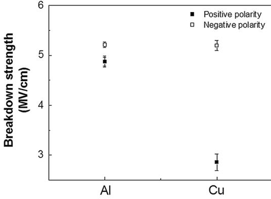
Fig. 4. Comparison of breakdown field for MIM capacitors with Cu and Al electrodes under positive and negative polarities.
