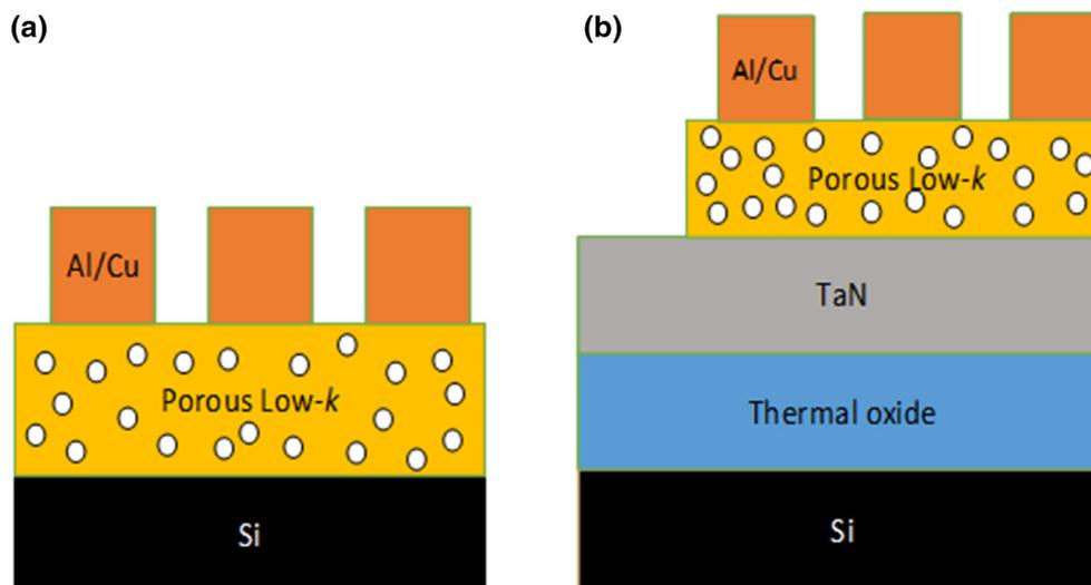
Fig. 1. Schematics of test structures employed in this study: (a) MIS and (b) MIM capacitor structures.
