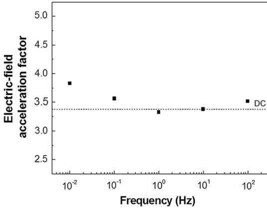
Fig. 8. Electric-field acceleration parameter of MIM capacitors with Cu electrode under bipolar AC stress as function of frequency.
