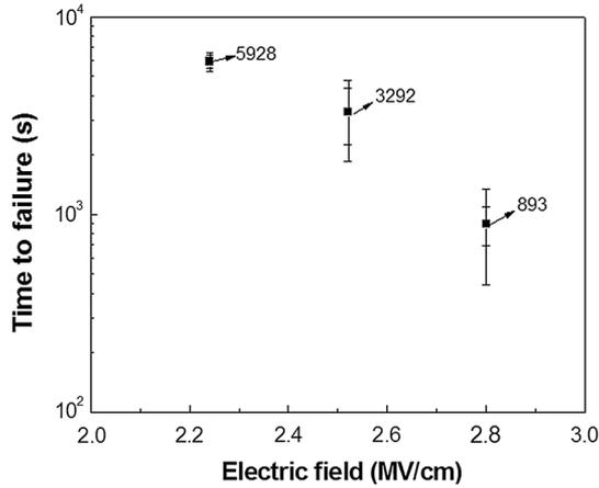
Fig. 6. TTF of MIM capacitors with Cu electrode under DC stress with positive polarity as function of electric field.
