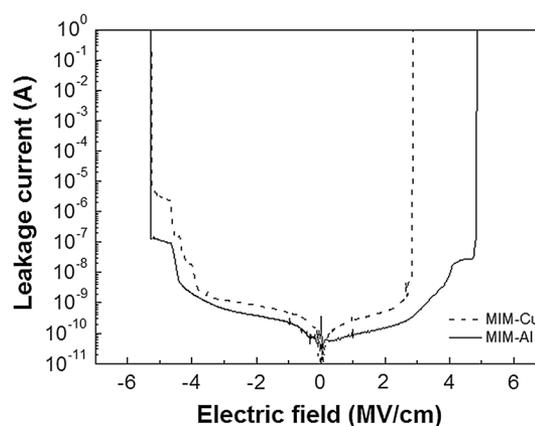
Fig. 3.  $I$ - $E$  characteristics of MIM capacitors with Cu or Al electrode.
