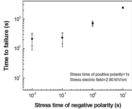
Fig. 9. TTFs of MIM capacitors with Cu electrode under bipolar AC stress as function of stressing time with negative polarity (stressing time in positive polarity = 1 s).
