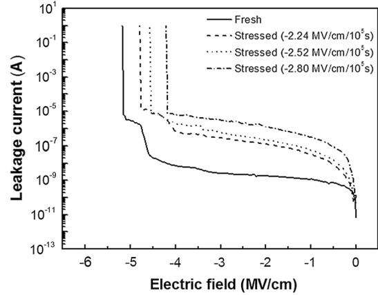
Fig. 5. Comparison of  $I$ - $E$  characteristics of fresh and stressed MIM capacitors with Cu electrode under stress with negative polarity.
