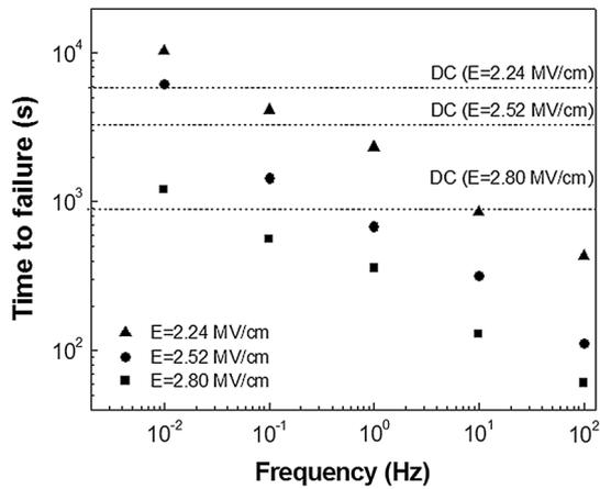
Fig. 7. TTFs of MIM capacitors with Cu electrode under bipolar AC stresses as function of frequency.
